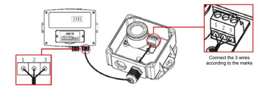
Wiring arrangement between OLC 10 TWIN and MX 15 control unit
