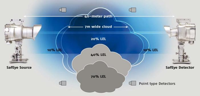
This scenario shows how the matrix of point type detectors can miss a leak or eventually only see diluted gas levels whereas SafEye 700S Open-Path will, in this case, measure  $20\% LEL \times 7 m = 1.4 LEL.m - well above 1 LEL.m alarm level$
